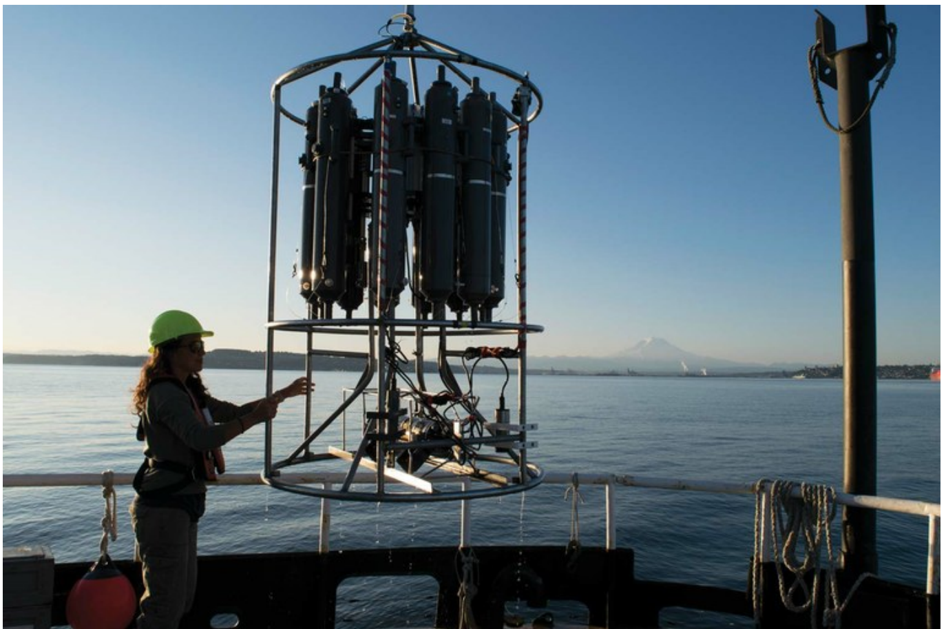
Aboard the research vessel affectionately known as Cliffy, researchers haul in the canisters and sensors that take readings as they collect samples in Puget Sound, Washington. – Courtesy Marine Lebec
