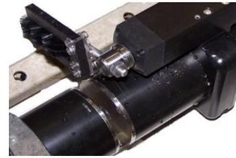
*Figure 2.13. The SUNA Hydro-Wiper.*
