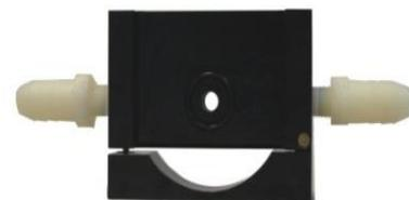
Figure 2.12. The SUNA flow cell.
